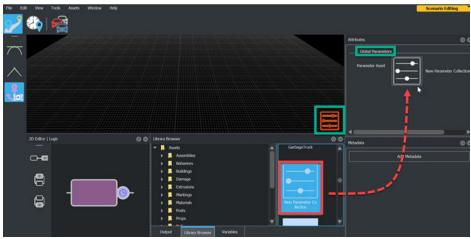
To assign a parameter collection to a scenario, drag the parameter collection asset from the **Library Browser** to the **Parameter Asset** field in the **Attributes** pane. You can set initial parameters by specifying their names in the corresponding **Name** fields and values in the corresponding **Value** fields.
